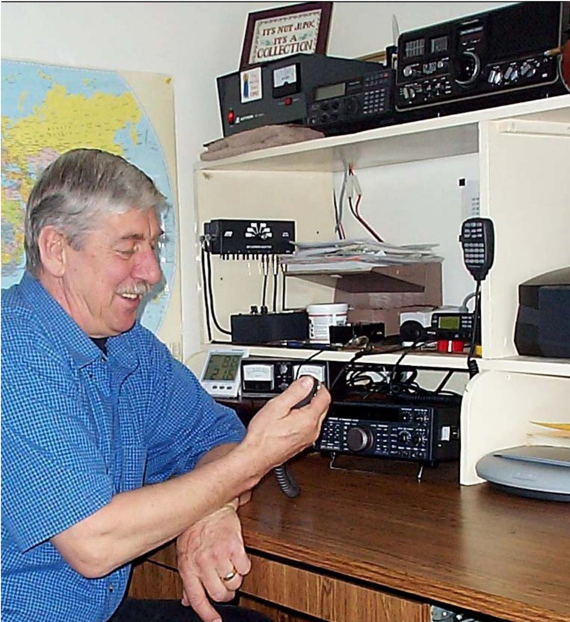
**John (VA5RJA) Station setup:- HF-** Kenwood TS450S, Astron RS35M Power supply. **2m-** Icom V8000. **Antennas-**G5RV and a 40-80m trapped dipole inverted V and an 80m horizontal loop to go up soon. Also a homemade J-Pole. **Mobile-**Icom 2100H to a 5/8 mag mount.
