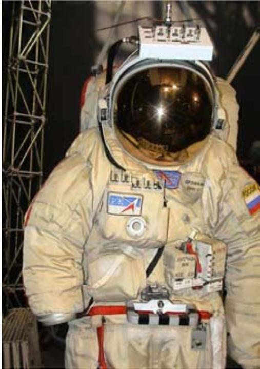
Now is the time to begin preparing your amateur radio station to receive signals from SuitSat, the most unusual Amateur Radio satellite ever orbited. SuitSat amateur radio equipment will be installed inside a surplus Russian Orlan spacesuit. It will become an independently orbiting satellite once it is deployed by the crew of the International Space Station during an extravehicular activity, tentatively planned around December 8, 2005.
