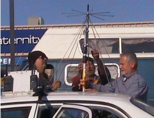
linking systems. Both cross band repeaters were standard off the shelf dual band mobiles connected to dual band antennas on push up masts attached to cars in parking lots. They operated throughout the exercise on battery power.
