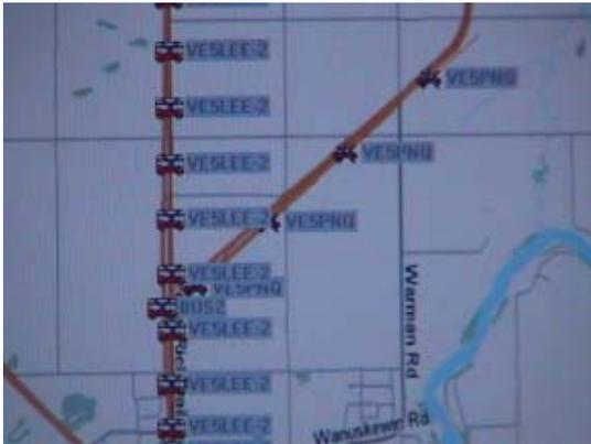
APRS was used to track the inbound evacuation buses and ARES vehicles heading for Martensville. APRS computers were located on the City of Saskatoon Command Bus, at the Saskatoon #9 Firehall EOC and the Martensville shelter allowing all 3 sites to see vehicle locations in real time.
